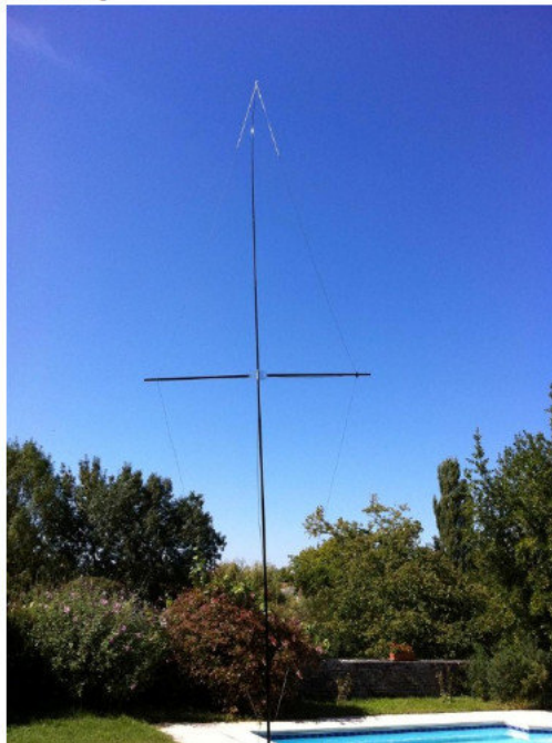
Step 7: Down side wires mounting
