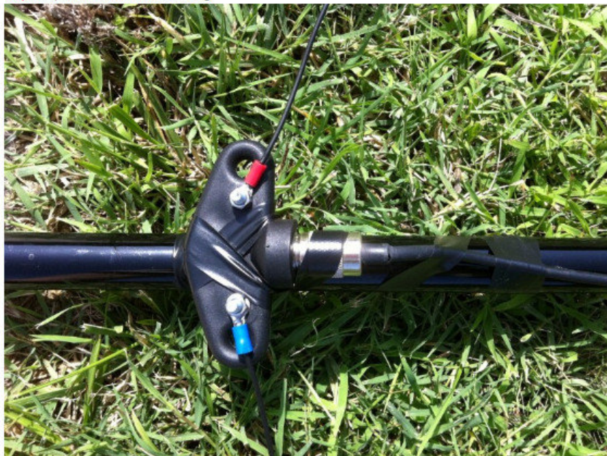
Step 2: Dipole & coaxial cable mounting
